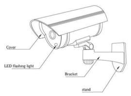
Once the batteries have been installed, the LEDs will blink at an interval of 3 seconds.
