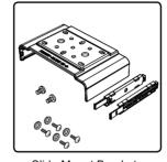
Slide Mount Bracket, Guide Rails and Screws
