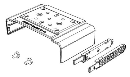
Align the guide rails along the side of the base and insert them into the slots provided. Then use the screws to lock them securely in position.
