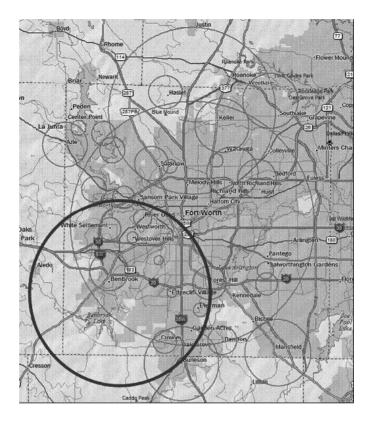
The scanner selects channels from systems that overlap the thick circle. So, the system down south that covers Burleson is included even though only part of it is covered, but Haslet, way up north, is not included.
